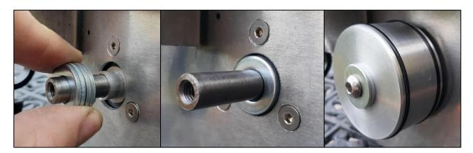
Always take care to hold the wheels while tightening or loosening the front bolts, as failure to do so can put undue strain on the internal gear mechanism. There is no need to over-tighten the front bolts.
